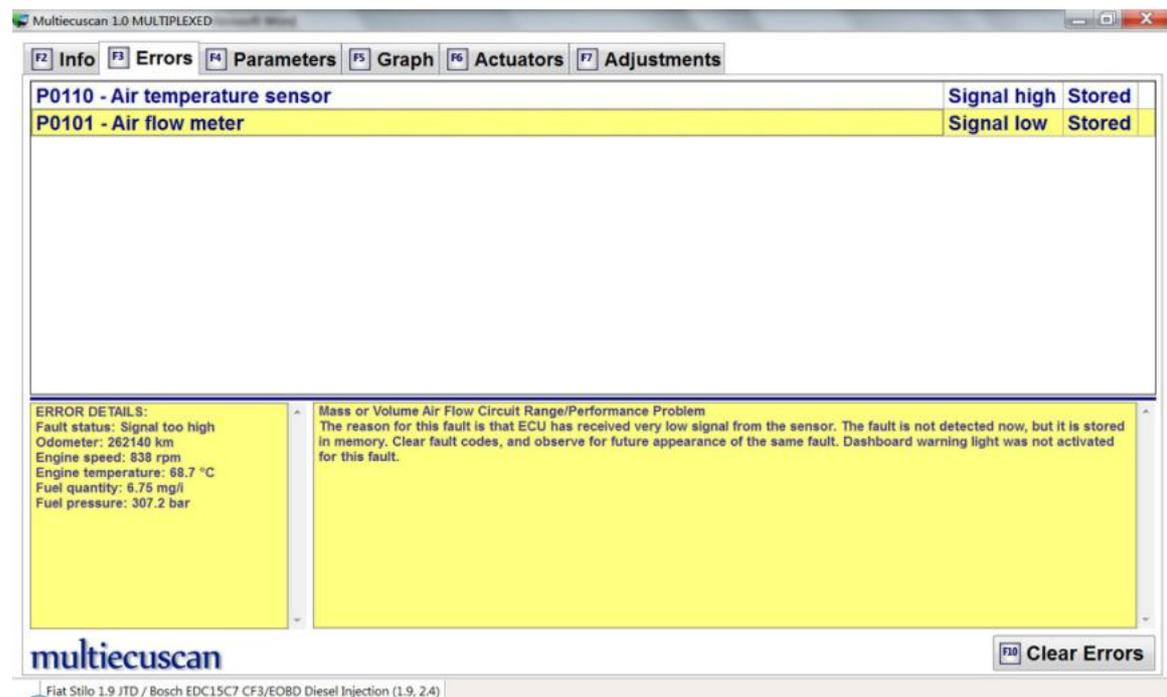
As you can see this control module reports 2 errors. Actually, I intentionally created these 2 errors by unplugging the MAF connector while the engine was working. In the lower left window you can see details about the conditions when the error code was detected.
